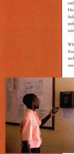
to the caching device using the infrared beam of their handheld units. The caching devices in turn communicate with a central server at the Ministry of Health (MOH) in Kampala via the GSM cellular network. Data collected in the field on a handheld computer can thus be uploaded to the caching device via infrared beam, stored on the cache until a regularly scheduled, off-peak call is initiated, then transmitted to the central server via the cellular network.
