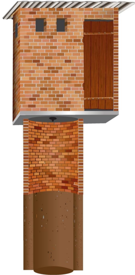
The transitional latrine includes a pit that is lined down to 1.5 meters to facilitate emptying.
